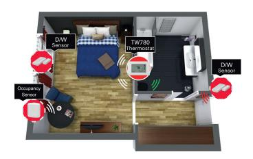
The TW780 EMS Kit includes a smart thermostat, and door/window and motion sensors.
